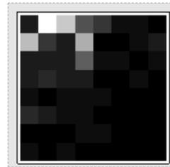
Quantized DCT of the example block.
